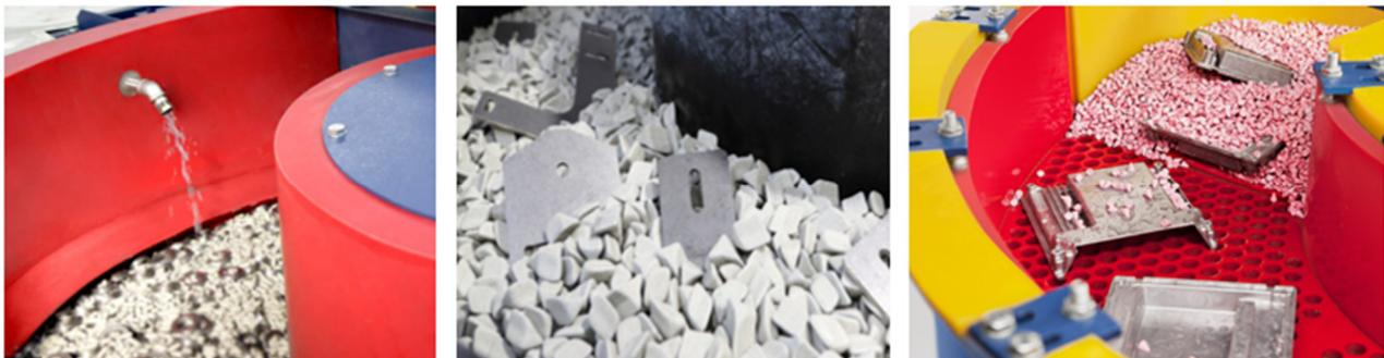
Exemplary illustration of the vibratory grinding of various components
